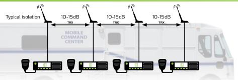
This communication solution is NOT recommended because the maximum isolation **without** one of Procom's mobile TX combiners PRO-ISO-PHY-TETRA-S is: 10-15 dB
