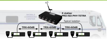
We recommend this communication solution because the maximum isolation with the mobile TETRA combiner PRO-ISO-PHY-TETRA-S exceeds 62 dB (TRX↔TRX)
