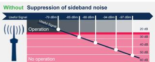
Many TETRA transmitters generate broadband TX sideband noise. The sideband noise is generated in the power amplifier. The sideband noise from one radio transmitter seriously degrade the sensitivity of a nearby positioned radio receiver. Depend-
