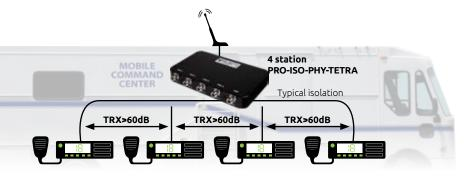
We recommend this communication solution because the maximum isolation **with** the mobile TETRA combiner PRO-ISO-PHY-TETRA-S **exceeds 62 dB** (TRX TRX)
